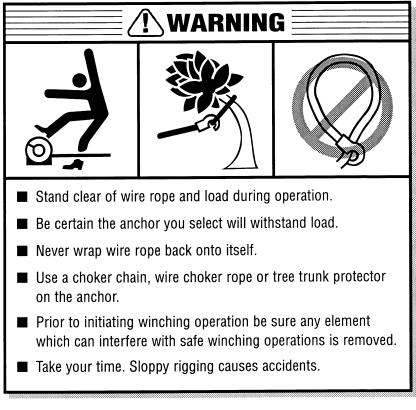
Always spool out as much wire rope as possible while leaving the last 5 wraps on the drum. Pick an anchor as far away as practical. This provides the winch with its greatest pulling power.
